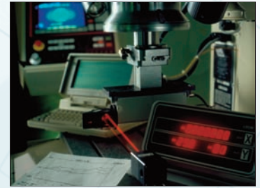
After final assembly, each machine is laser tested in NASA's quality control center.
